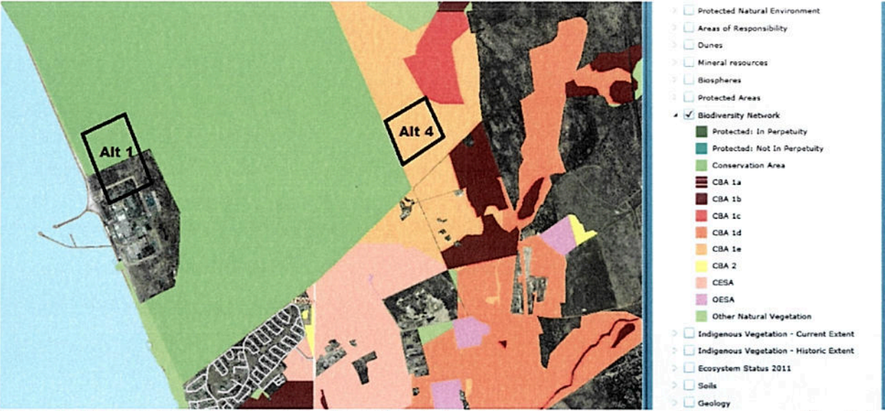
Figure 2: Diagram indicating the two alternatives being taken through into the EIA phase and its relation to the BioNet Critical Biodiversity Area (CBA) layer.
